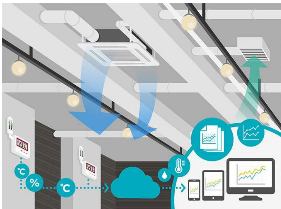
Figure 6. Working of HVAC System Control.
