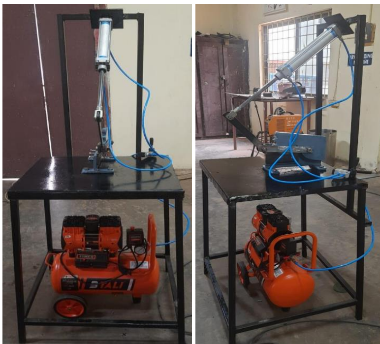
Figure 16. Final setup of pneumatically actuated sheet metal cutting machine.
