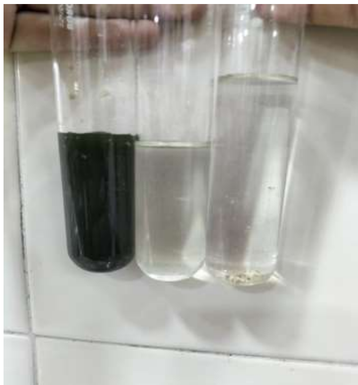
Figure 12. Wastewater, nano solution and treatment [showing accumulation of solid waste particles].
