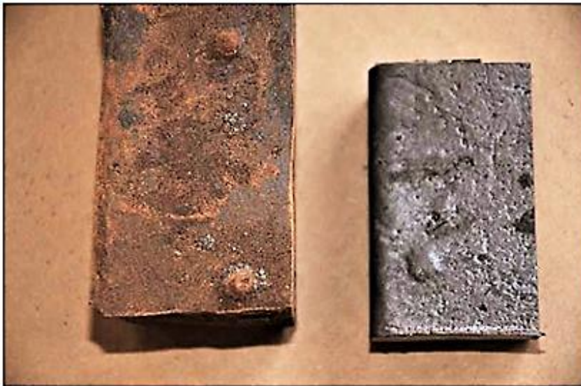
Figure 12: Ductile iron casting surface. On the left side, a casting made in the "in-mold" technology. On the right, the casting surface is made in the traditional sandwich spheroidization method
