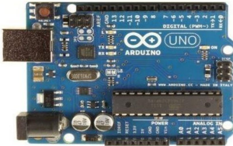
Figure 3. Arduino board with In-circuit Serial Programming (ICSP).
