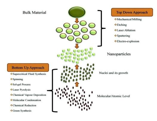
Fig. 1 Synthesis approaches of nanoparticles
