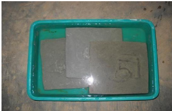
Figure 6. Water absorption test.
