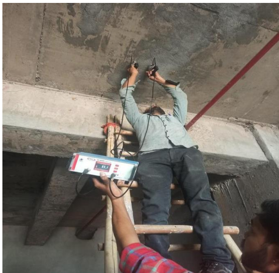
Figure 1. Ultra sonic pulse velocity test (upv).
