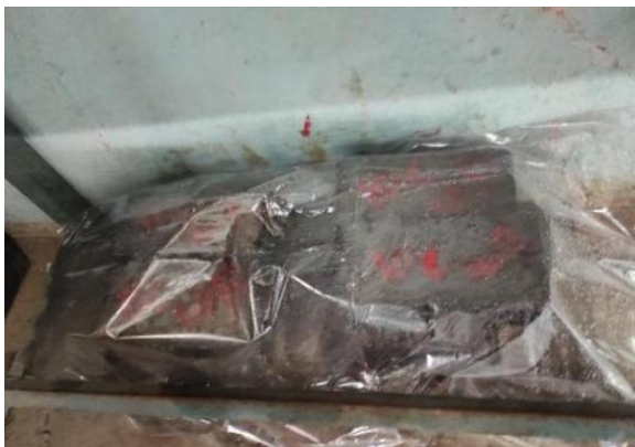
Figure 4. Curing of blocks.
