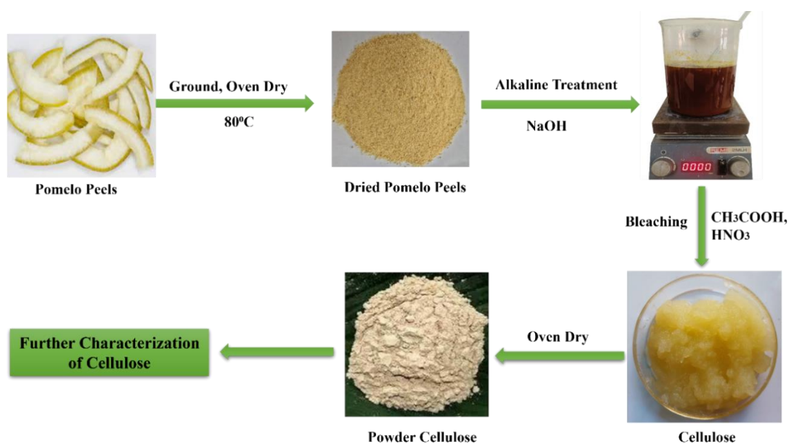
Figure 2. Flow chart of synthesis of nanocellulose from pomelo peels.
