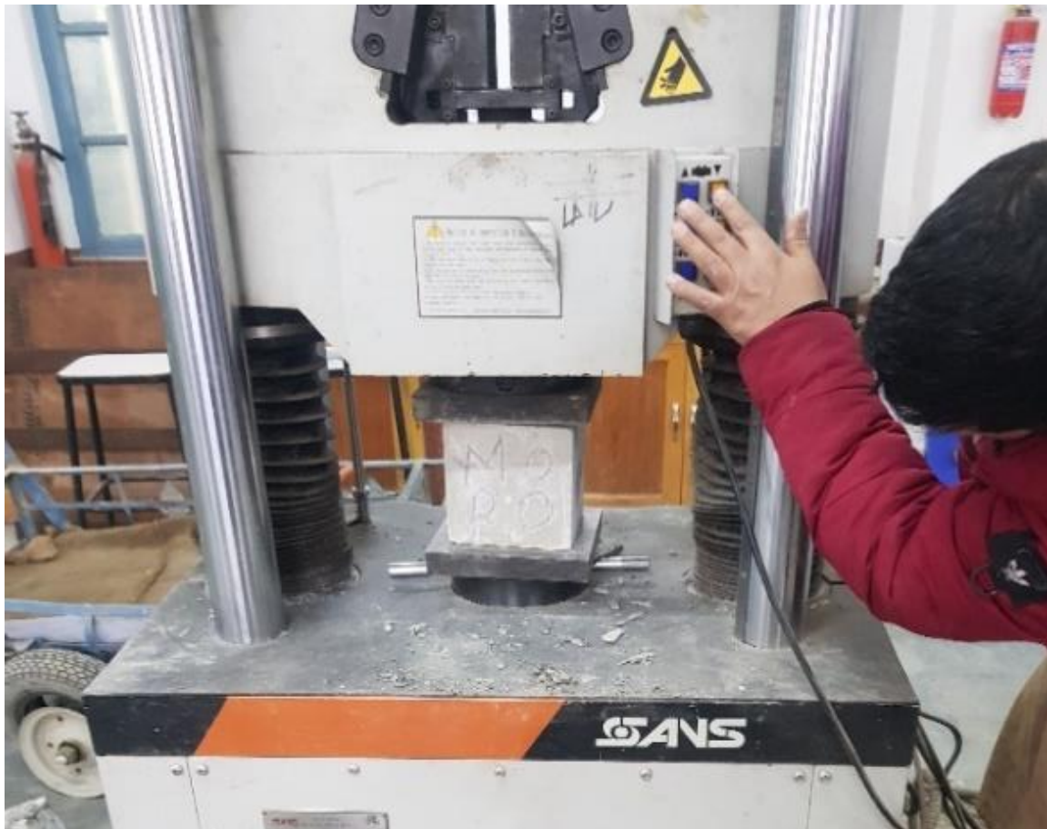
Figure 2. Compressive strength testing setup.
