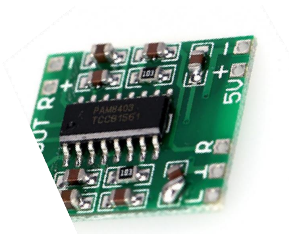
Figure 3. Amplifier used in bus stop reminder.
