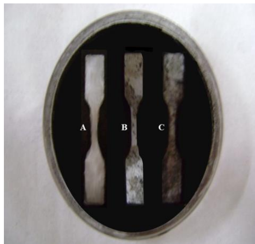
Figure 5. Sample degradation following Pseudomonas aeruginosa exposure: (A) virgin LDPE, (B) LMS 30A , and (C) LUS 30 composites.
