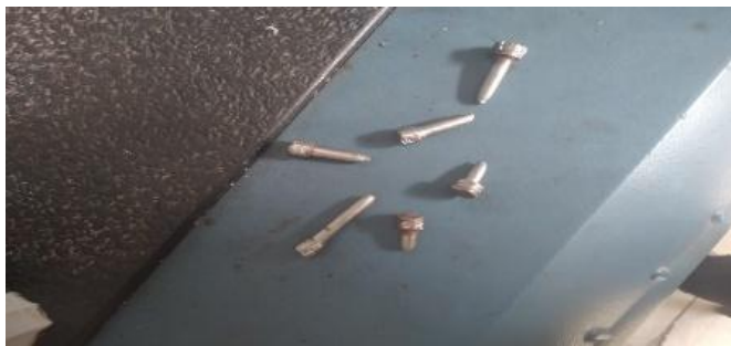
Figure 3. Samples after tensile test was carried out.
