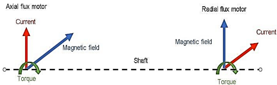
Figure 4. Compression of current and magnetic flux in radial-flux and AFM [13].
