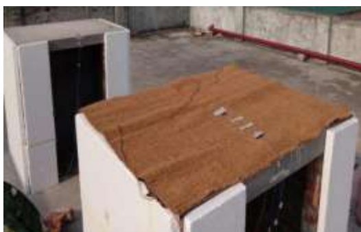
Figure 1. Experimental set up with dry coir mat and perlite [12].
