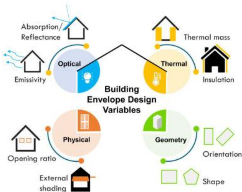
Figure 1. Various type of building envelope design variables.
