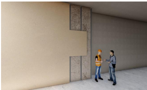
Figure 5(c). Eutectic PCM can be incorporated inside the drywall for use in interior walls which makes it less costly and has high thermal storage as compared to conventional walls.
