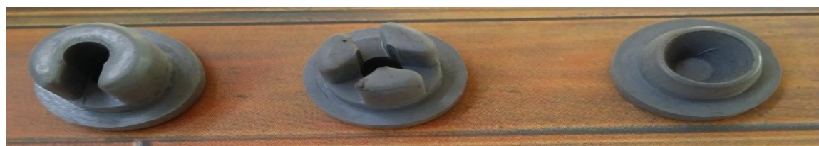
Figure 5. Pharmaceutical stopper made of bromobutyl phosphonium ionomer.
