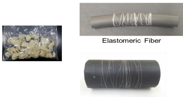
Figure 8. Elastomeric fibers from ammonium ionomer based on 4-DMAP.
