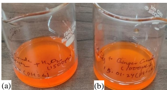
Figure 4. MO reaction solutions (a) MO solution in pH 6 + ginger juice + H 2 O 2 and (b) MO solution in pH 6 + ginger juice.
