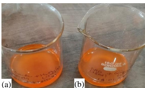
Figure 5. MO reaction solution (a) MO solution in pH 8 + ginger juice + H 2 O 2 and (b) MO solution in pH 8 + ginger juice.
