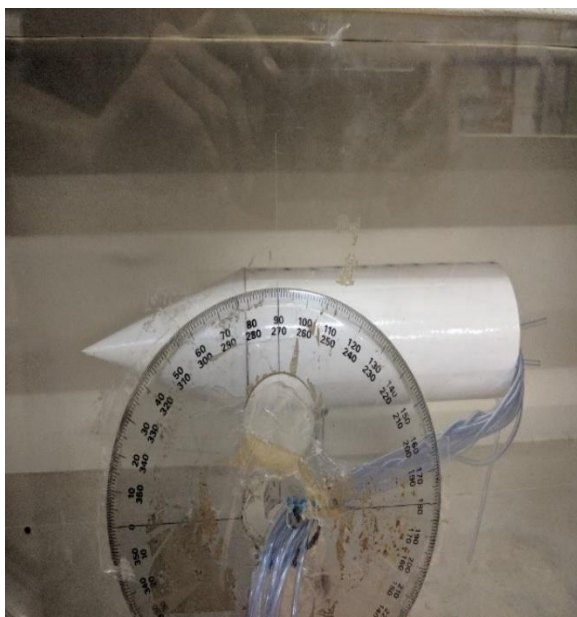
Figure 5. Experimental setup of cylindrical mid-section with power series1 forebody.
