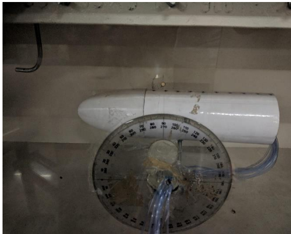
Figure 6. Experimental setup of cylindrical mid-section with power series 0.25 forebody.
