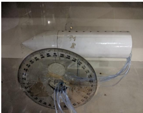
Figure 7. Experimental setup of cylindrical mid-section with secant ogive forebody.
