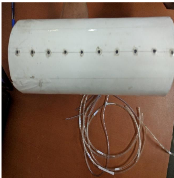
Figure 4. Cylindrical mid-section body with 10 holes.
