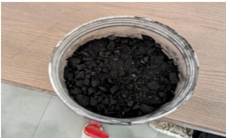
Figure 6. Layer 5: 4 cm thick biochar layer (4–10 mm).
