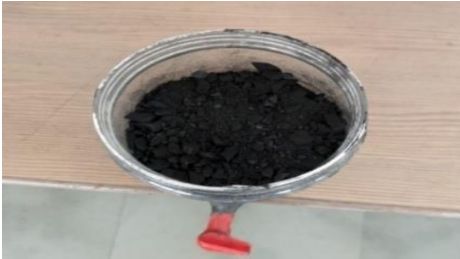
Figure 4. Layer 3: Biochar layer: 3 cm thick (<4 mm).
