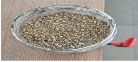
Figure 3. Layer 2: Sand layer: 2 cm thick (<4 mm).
