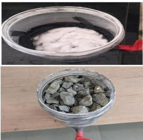
Figure 7. Layer 6: Topmost layer of gravel size 10–20 mm.
