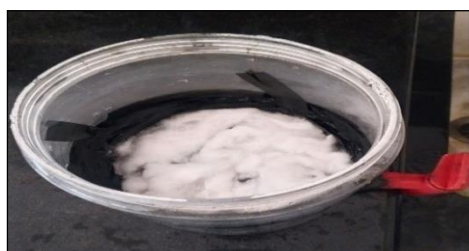
Figure 2. Layer 1: Cotton layer: 1 cm thick.
