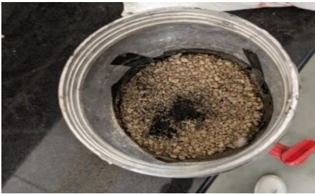
Figure 5. Layer 4: 2 cm thick sand layer (<4 mm).
