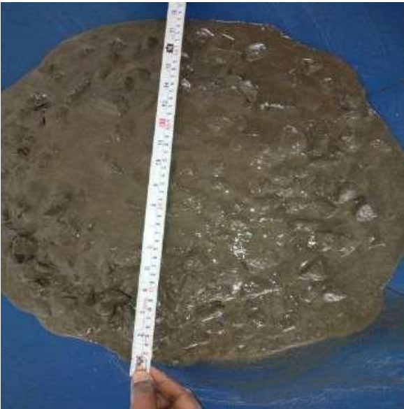
Figure 6. Flow test. Flow Percentage = 60%.
