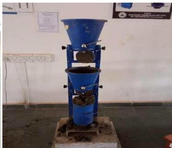
Figure 5. Compaction factor test. Compaction Factor Value = 0.95.
