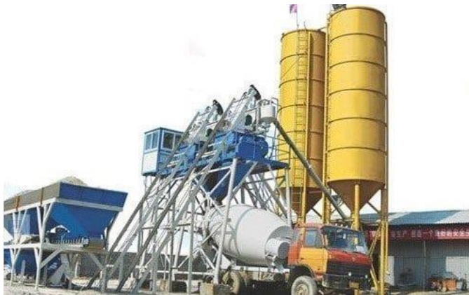
Figure 1. RMC batching plant.
