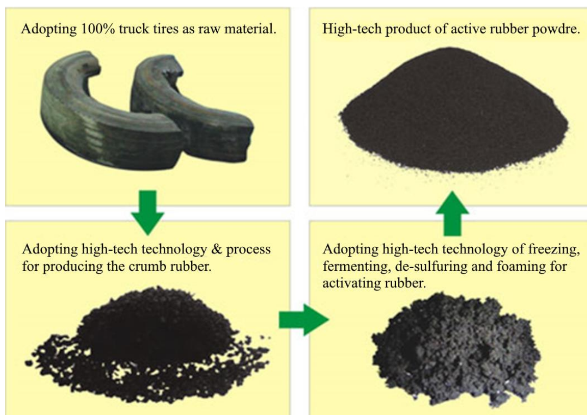
Figure 1. Typical powder production process of rubber powder from end-of-life tires.
