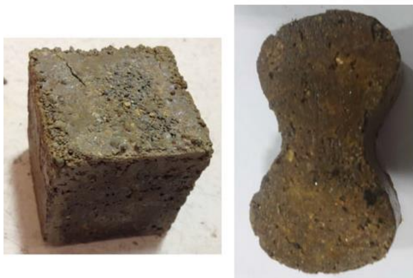
Figure 11. Molded concrete products from sulfur-based copolymer [36].
