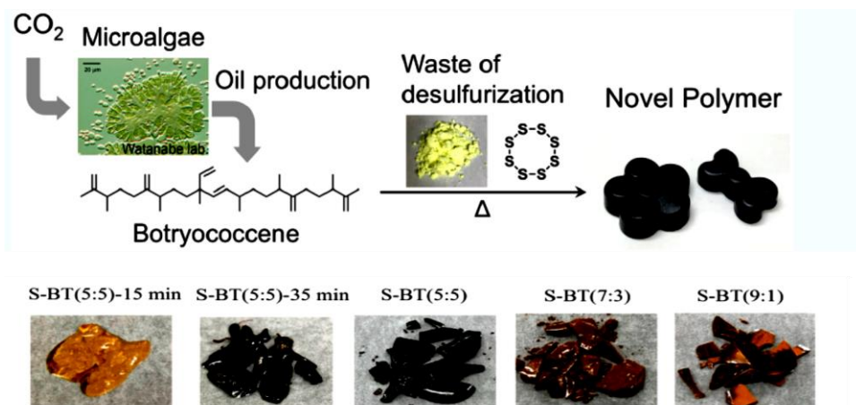
Figure 2. Sulfur copolymer from algae Botryococcus braunii and elemental sulfur [25].
