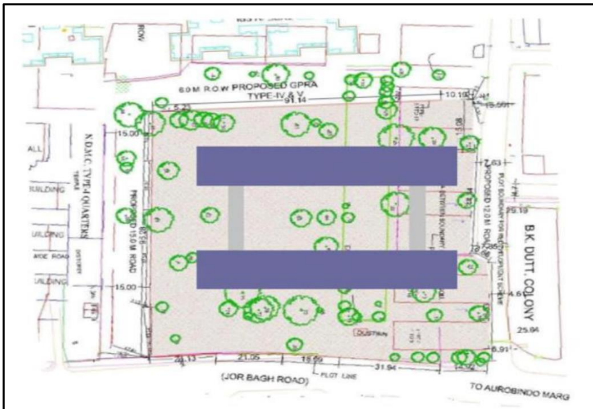
Figure 4. Final design view of North-South blocks orientation and courtyard (Indira Paryavaran Bhawan Redevelopment Plan, New Delhi).
