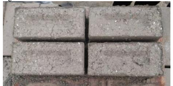
Figure 5: - Plastic bricks after 28 days of curing, prepared for strength testing.
