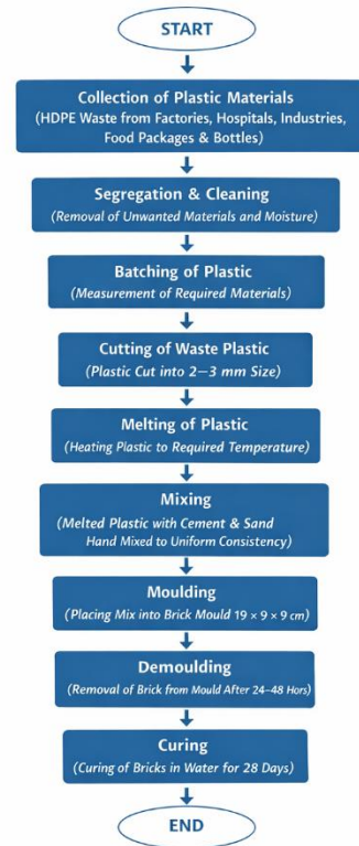
Figure 1: - Flowchart of the proposed methodology for plastic brick production.
