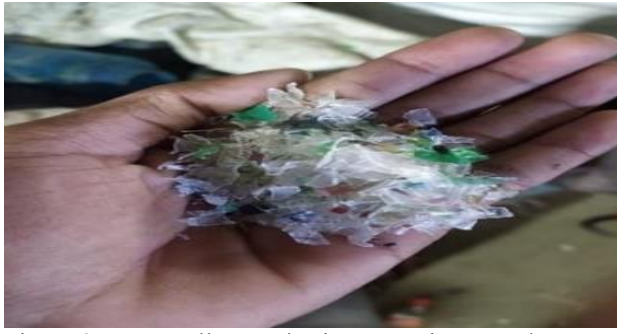
Figure 2: - Manually cut plastic waste pieces ready for mixing in brick production.
