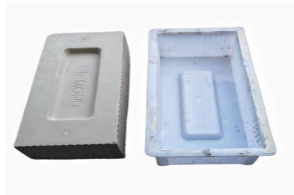
Figure 4 :- Brick mould used for shaping the prepared plastic-cement mixture.
