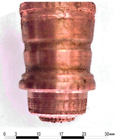
Figure 7. Copper version of the sample geometry, machined with coolant and adjusted parameters.
