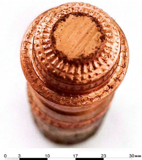
Figure 9. Close-up of copper base showing concentric toolmarks from discrete angular indexing.
